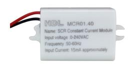
HDL-MCR01.40 is a TRIAC constant current load, the module can supply minimum current for TRIAC. It can solve the flicker problem when it is dimming the lamps, such as LEDs and electronic transformer.
